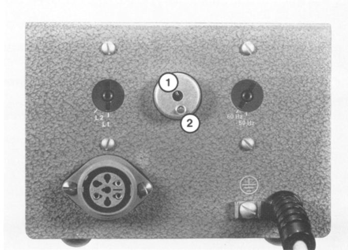
Fig. 6 Transformer for the 50W high-pressure mercury lamp
